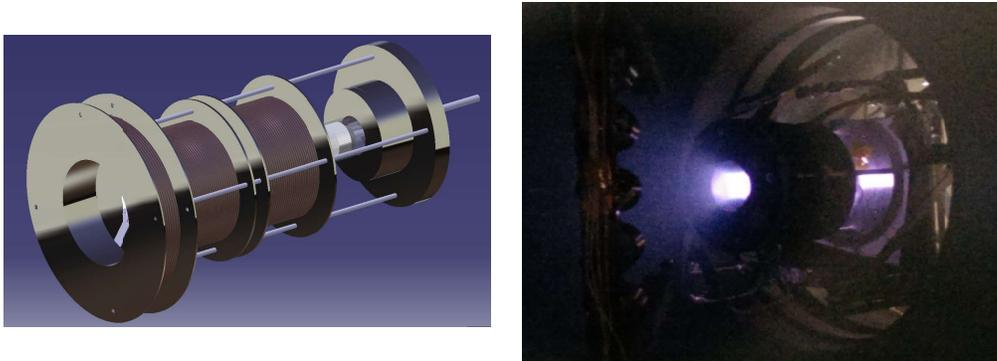
Figure 1. Left: CAD draw of the HPT05 prototype [Ref. 16]. Right: HPT05 prototype under testing at Corona vacuum chamber, ESA-ESTEC [Ref. 17].
