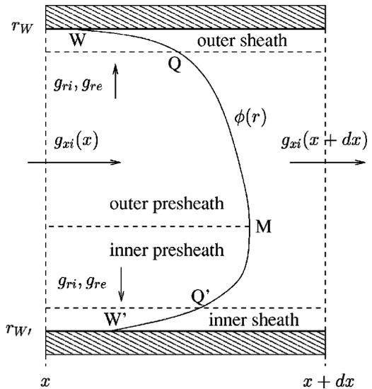
FIG. 1. A generic radial section of a long annular channel between two dielectric walls.  $g_{xi} = n_{xi} v_{xi}$  and  $g_{ri} = n_{ri} v_{ri}$  represent axial and radial particle fluxes;  $\phi(r)$  sketches the radial profile of the electric potential, which is maximum at point  $M$ . The transitions to the sheaths are at points  $Q$  and  $Q'$ . Since the presheath/sheath structure corresponds to the zero Debye-length limit one has  $r_w = r_Q$  and  $r_{w'} = r_{Q'}$ .
