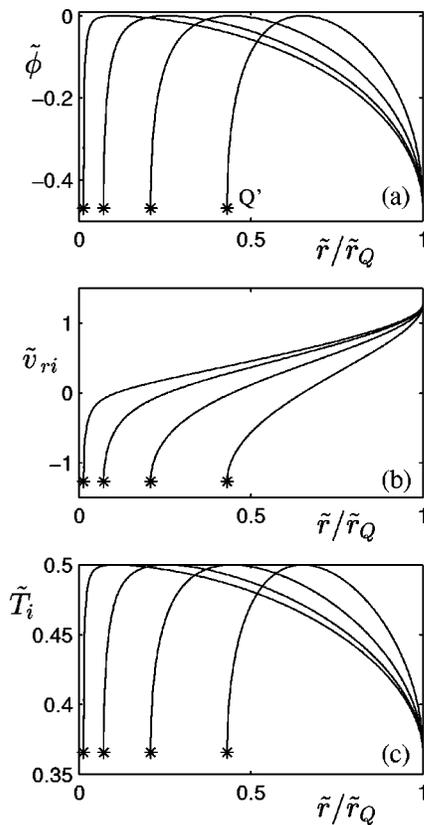
FIG. 5. Annular geometry: Plasma profiles for different annular ratios ( $r'_Q/r_Q=0.013, 0.072, 0.21, 0.43$ ),  $\tilde{T}_{iM}=0.5$ , and  $\tilde{\nu}_r=\tilde{\nu}_i=0$ . Points  $Q'$  are at the asterisks; points  $M$  are at  $d\phi/dr|_M=0$  (and  $\tilde{\nu}_{ri}=0$ ) separating the inner and outer presheaths.
