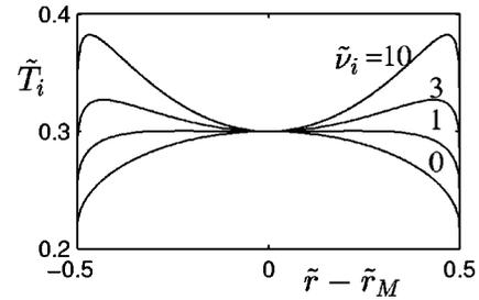
FIG. 4. Planar geometry: Radial profiles of the ion temperature for  $\tilde{T}_{iM} = 0.3$ ,  $\tilde{\nu}_r = \tilde{\nu}_i$ , and four ionization frequencies:  $\tilde{\nu}_i = 0, 1, 3,$  and 10.
