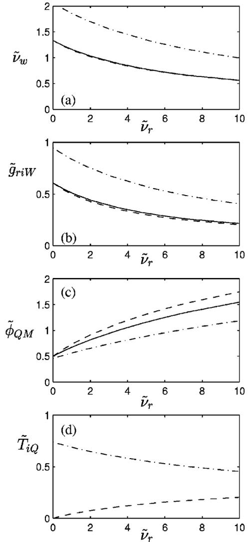
FIG. 2. Planar geometry: Evolution of plasma parameters with  $\tilde{v}_r$  for  $(\tilde{T}_{iM}, \tilde{v}_i) = (0,0)$  [solid line],  $(1,0)$  [dashed-dotted line], and  $(0, \tilde{v}_r)$  [dashed line]. The dimensionless particle flux is  $\tilde{g}_{ri} = (n_{iM} \sqrt{T_e/m_i})^{-1} g_{ri}$ .
