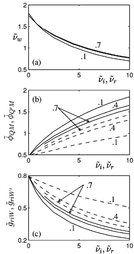
FIG. 6. Annular geometry: Evolution of main plasma parameters with  $\tilde{\nu}_i$  for  $\tilde{T}_{iM}=0.5$ ,  $\tilde{\nu}_r=\tilde{\nu}_i$  and three annular ratios,  $\beta=0.1, 0.4$ , and  $0.7$ . In (b) and (c) solid lines correspond to the outer presheath, and dashed lines to the inner presheath.
