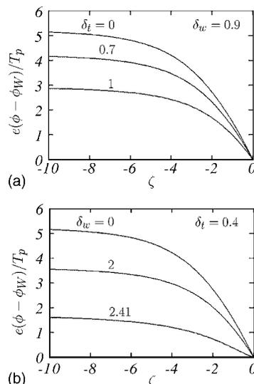
FIG. 2. Sheath solution. Profiles of the electrostatic potential for (a)  $\delta_w = 0.9$  and several values of  $\delta_t$  from 0 to 1; (b)  $\delta_t = 0.4$  and several values of  $\delta_w$  from 0 up to the charge-saturation limit.
