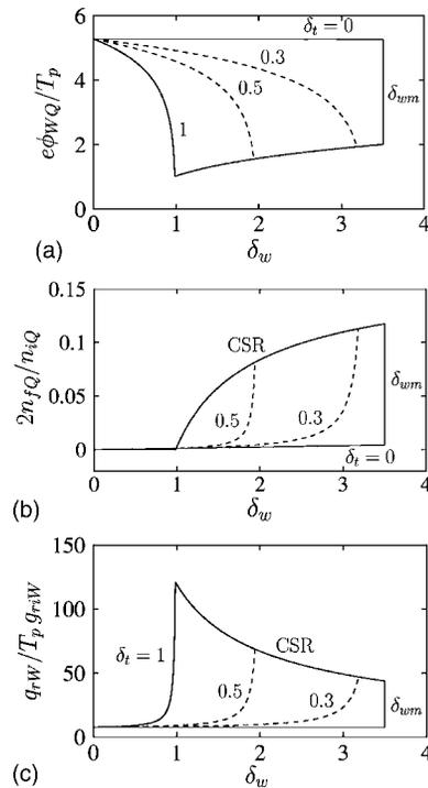
FIG. 5. Parametric region of solutions, in terms of  $\delta_w$  and  $\delta_t$ , for (a) the sheath potential drop, (b) the density of free secondary emission at point  $Q$ , and (c) the radial losses of energy. The limits are zero-trapping, total-trapping, charge-saturation, and maximum SEE yield (here  $\delta_{wm}=3.5$ )
