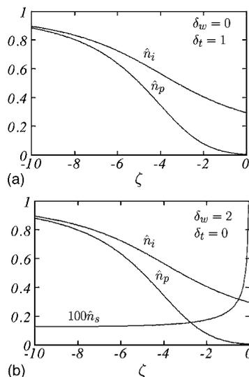
FIG. 3. Sheath solution. Profiles of the densities of the different species for (a)  $\delta_w = 0$ , and (b)  $\delta_w = 2$  and  $\delta_t = 0$ . In this and next figures  $\hat{T}_{iQ} = 0$ . Notice that  $n_f = n_s$ , and the curves are plotted 100 times these densities. In the sheath scale the presheath is at  $\zeta_Q = -\infty$ .
