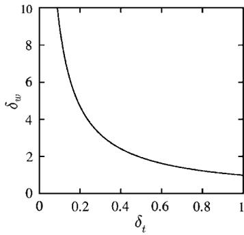
FIG. 4. SEE yield vs the trapped fraction at the charge-saturation limit.
