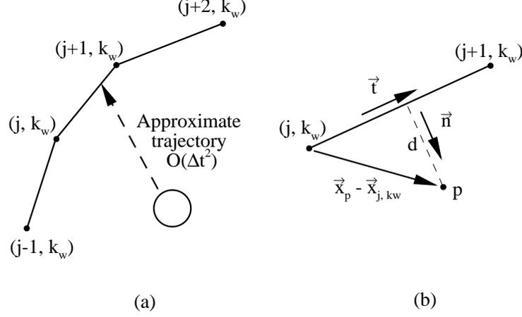
**Figure 2.** (a) Sketch of the impact of a macroparticle with the boundary. (b) Distance to the boundary.
