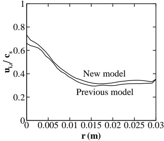
Figure 5. Velocity perpendicular to the outer wall divided by the Bohm velocity ( $c_s = \sqrt{T_e/m_i}$ ) in different axial positions of an SPT-70 type Hall thruster.
