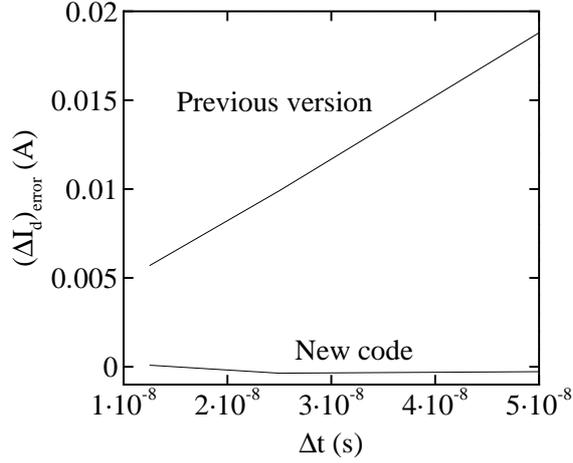
Figure 4. Comparison of the error in the current through the Hall thruster between a previous version and the new code.
