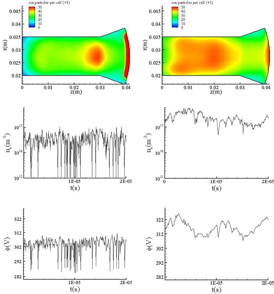
Figure 6. Comparison between HPHall-2 (left column) and the new hybrid simulation code (right column): Contour Number of macroions per cell, temporal evolution of plasma density and potential in a node of the anode sheath edge.
