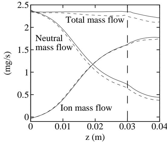
Figure 3. Mass flows in a SPT-70 like simulated Hall thruster computed by HPHall (dashed lines) and the new algorithms (solid lines).
