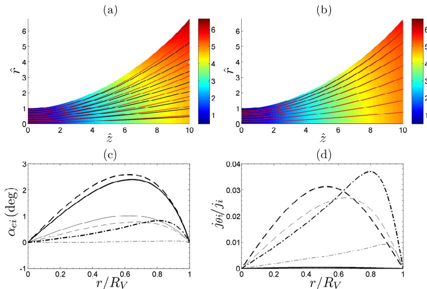
**Figure 3.** (a)-(b) Ion(black) and electron/magnetic(red) streamlines in the meridional plane for  $\hat{\Omega}_{i0} = 0.1$ (a) and 100 (b); the color 2D map plots the ion velocity  $\hat{u}_i$ . (c) Misalignment angle between ion and electron streamlines and (d) relative azimuthal ion current, at  $z/R = 5$ (thin lines) and 10 (thick lines) for  $\hat{\Omega}_{i0} = 0.1$ (solid), 10(dashed), and 100(dash-and-dot).
