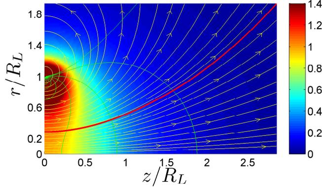
Figure 1. Magnetic streamlines and magnetic strength (in color, arbitrary units) for a circular ring of radius  $R_L$ . The red line corresponds to the boundary  $V$  of the plasma jet in the nozzle used in the simulations.
