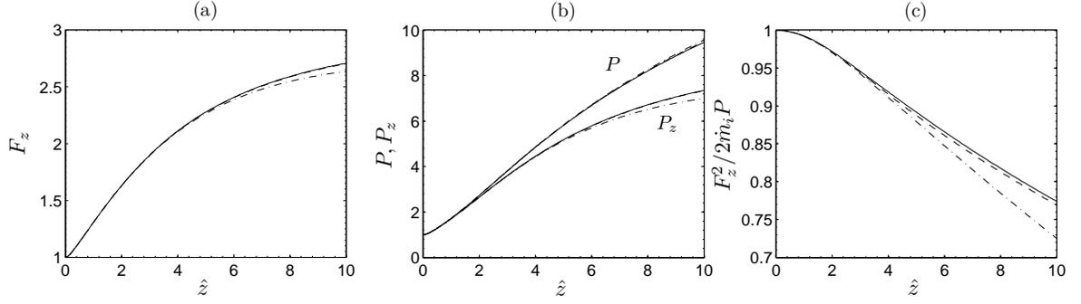
Figure 6. Axial evolution of ion (a) thrust, (b) axial and total power, and (c) acceleration efficiency, for  $\hat{\Omega}_{i0} = 0.1$ (solid), 10(dashed), and 100(dash-and-dot).
