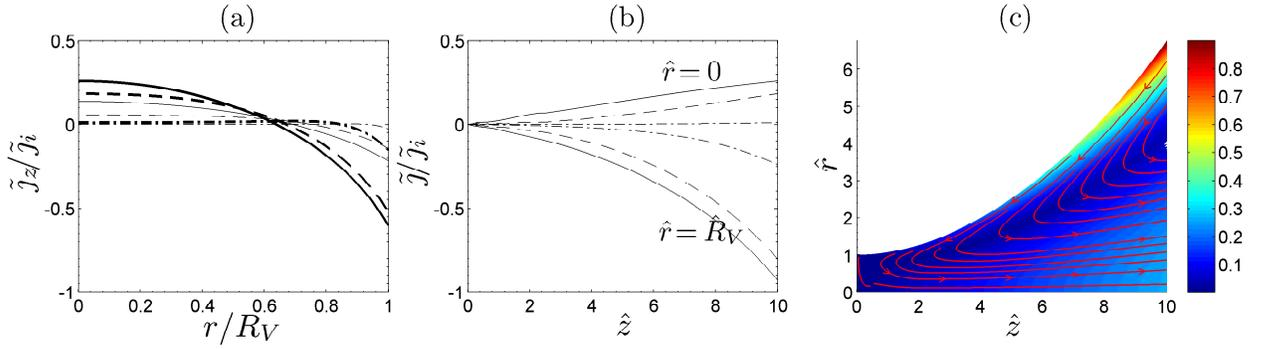
Figure 4. (a) Relative electric current along  $z$  for same conditions than Figs.3(c) and 3(d). (b) Relative electric-current for same conditions than Fig. 2. (c) Lines of electric current density and (in color)  $|j|/j_i$  for  $\hat{\Omega}_{i0} = 0.1$ .
