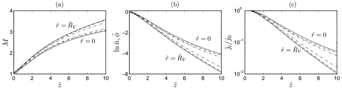
**Figure 2.** Axial evolution of plasma magnitudes at the two boundary streamlines,  $r = 0$  and  $r = R_V(z)$ , for three magnetization strengths:  $\hat{\Omega}_{i0} = 0.1$  (solid), 10 (dashed), and 100 (dash-and-dot).
