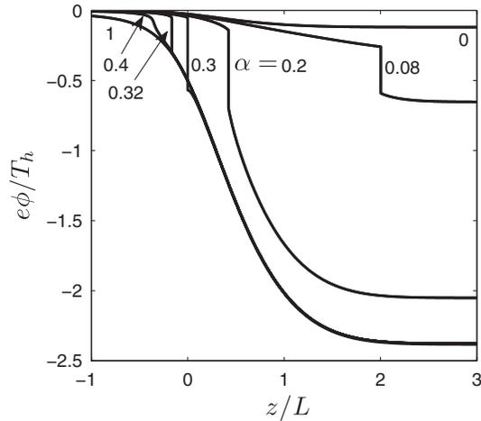
FIG. 4. Changes in plasma profiles and DL location with the density ratio for  $\tau = 20$ , several  $\alpha$ , and the nozzle profile  $A(z)/A_S = 3 - 2\exp(-z^2/L^2)$ ; the throat is at  $z = 0$ .
