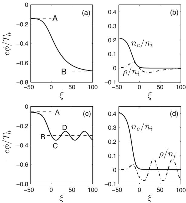
FIG. 3. Internal structure of a DL located in (a)–(b) the divergent side [ $\tau = 20$ ,  $\alpha = 0.20$ ], and (c)–(d) the convergent side [ $\tau = 20$ ,  $\alpha = 0.32$ ]. Dashed lines correspond to entrance  $A$  and exit  $B$ . These DL inner profiles are seen as discontinuities in the quasineutral profiles of Fig. 4.
