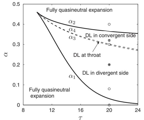
FIG. 2. Solid lines,  $\alpha_1(\tau)$  and  $\alpha_2(\tau)$  bound the parametric region where a DL is formed. Dashed lines,  $\alpha_3(\tau)$  and  $\alpha_4(\tau)$ , bound regions with different DL types. Asterisks correspond to the DL profiles shown in Fig. 3. Open circles correspond to the plasma profiles shown in Fig. 4.
