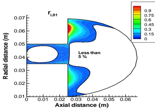
Figure 13. Ratio  $r_i$  of the ion production 0-1 by secondary electrons.
