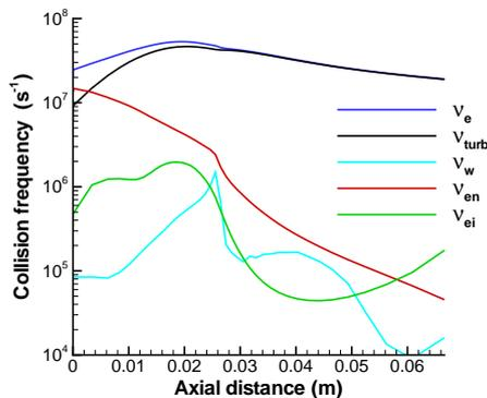
Figure 3. Typical collisional frequencies in our simulations of the SPT-100 Hall thruster.
