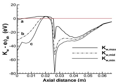
Figure 11.  $K_w - e\phi_{sh}$  at the outer wall of the thruster for the three cases of incidence of the secondary electron into the sheath.
