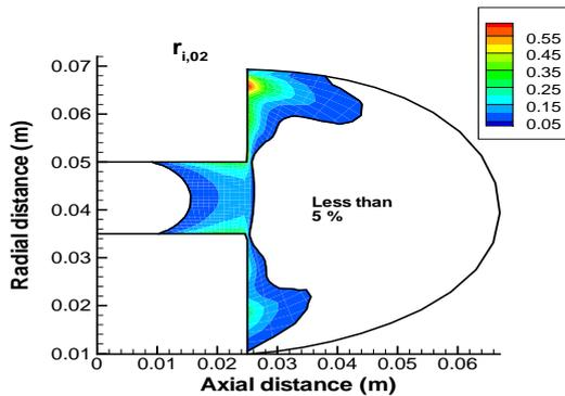
Figure 14. Ratio  $r_i$  of the ion production 0-2 by secondary electrons.
