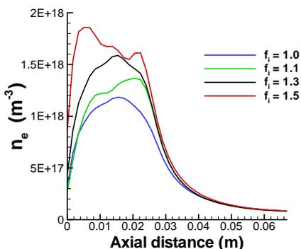
Figure 4. Density profiles of simulation 2.
