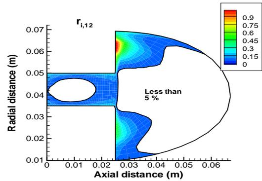
Figure 15. Ratio  $r_i$  of the ion production 1-2 by secondary electrons.
