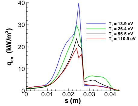
Figure 10. The electron energy flux to the outer wall of the thruster for simulation 5.
