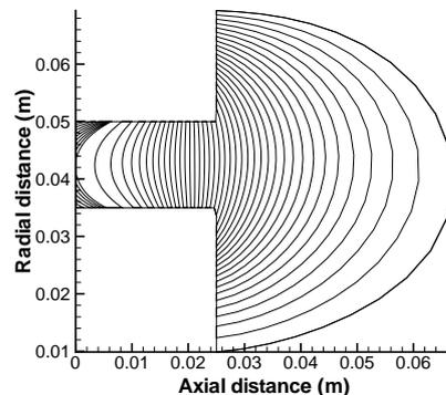
Figure 2. Magnetic field lines of the SPT-100 Hall thruster.
