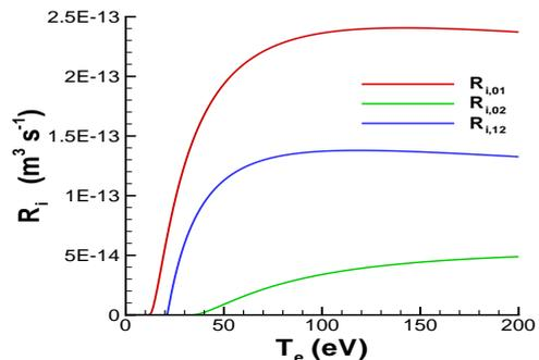
Figure 12. Ionization rates for secondary electrons.
