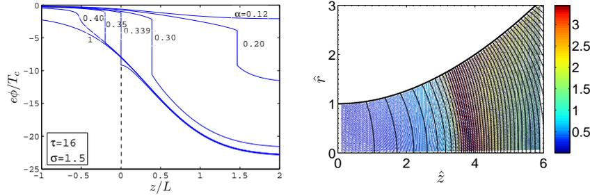
Figure 6: (Left) QSL and DL formation in an expanding plasma from the quasi-1D model;  $\alpha$  is the upstream hot-to-cold electron ratios for density and temperature, respectively;  $\sigma$  characterizes the nozzle expansion area. (Right) Maps of the ambipolar electric field and equipotential lines, illustrating the presence of a QSL from the 2D nozzle for  $\tau = 9$ .
