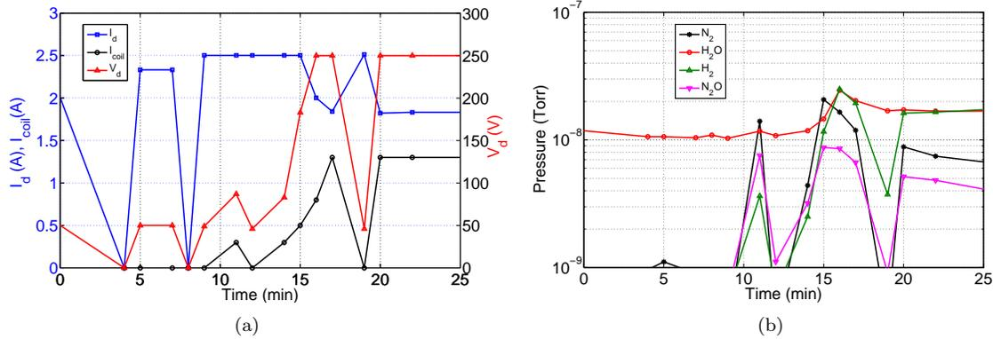
**Figure 4.** Anode experiment. The magnetic field is gradually increased during the plasma discharge. (a) The current-voltage curve of the experiment.  $I_{coil}$  is the current of the magnetic coils. (b) The pressure traces of the impurities.
