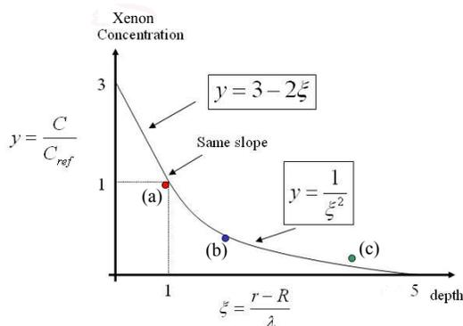
**Figure 1. Dimensionless concentration of Xenon inside the boron nitride walls of the thruster. Reference parameters are:  $C_{ref} = 0.0074$  and  $\lambda = 80$  nm. Dots in the figure represent experimental values from reference:<sup>7</sup> (a)  $y = 1$  and  $\xi = 1$ , (b)  $y = 0.2568$  and  $\xi = 2$ , and (c)  $y = 0.1622$  and  $\xi = 4.25$ .**
