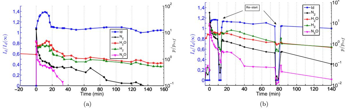
Figure 2. Transitional regime of experiment 1. Discharge current with different residual gas traces.  $I_d(\infty) = 1.68(A)$ ,  $p_{ref} = 10^{-8} \text{ torr}$ . (a) Typical behavior of the transitional regime. (b) Transitional regime with re-start up processes. The history is recovered.
