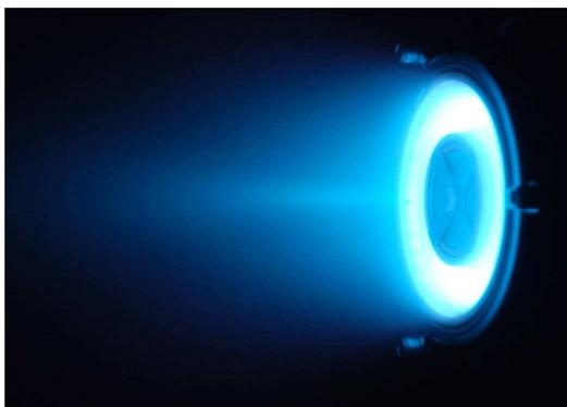
Figure 3. The 200 W-class PPI HET operating at 200 V and 1.0 mg/s in the NExET test bench (side view).
