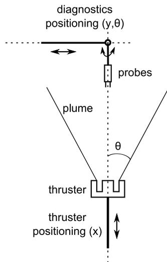
Figure 2. Schematic view of the HET and probe positioning system.
