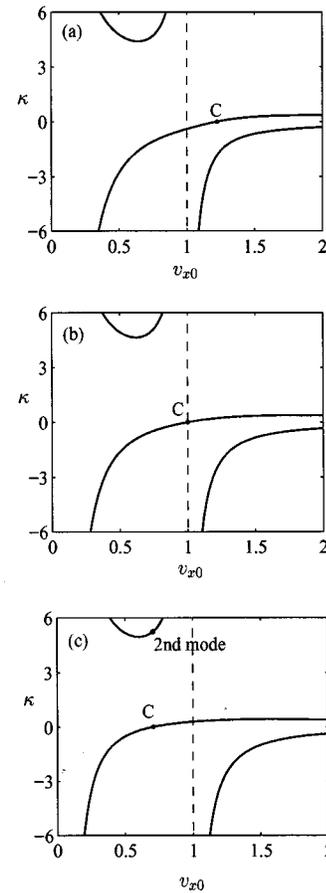
FIG. 9. Solutions of the dispersion relation for  $\Lambda_{dm}=1$ ,  $t_r=1$ , and  $\psi$  (in degrees) = 30(a), 45(b), and 60(c). At  $v_{x0} = v_{xC}$ ,  $\kappa=0$  is always a solution and yields a potentially evanescent mode; only in case (c), a second (exponentially) evanescent mode sets in.
