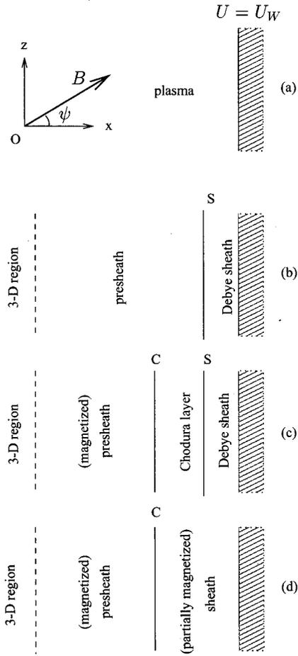
FIG. 1. (a) Reference frame used in the model and angle of incidence of  $\mathbf{B}$ ;  $Oxz$  is the plane of incidence. Sketches of the plasma structure for (b) weak, (c) intermediate, and (d) strong  $B$  field. In each case, the transition points, C or S, marked in the figures are well defined: they are singular/sonic points of the plasma equations. The transition to the 3-D region, not discussed here, is not well defined in the 1-D model.
