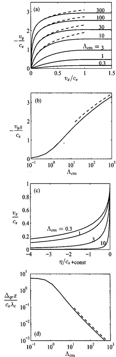
FIG. 5. Weak  $B$  field:  $\Lambda_{cm} = O(1)$  and  $\Lambda_{dm} = 0$ . Plasma response for  $\psi = 90^\circ$ . Dashed lines correspond to the approximate solution (24). In (d)  $\Delta_{qr}x$  represents the distance between  $\phi = \phi_S$  and  $\phi = \phi_S - 2t_r$ .
