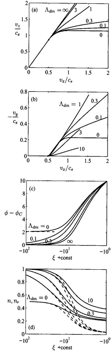
FIG. 6. Strong  $B$  field:  $\Lambda_{cm} \rightarrow \infty$ ,  $\Lambda_{dm} = O(1)$ . Plasma response for  $\psi = 60^\circ$ ,  $t_r = 3$ ,  $\phi_w \leq 10$ , and  $\Lambda_{dm} = 0$  (intermediate- $B$  case), 0.1, 0.3, 1, 3, 10, and  $\infty$ . Point  $C$ , separating presheath and sheath, is marked by a dot. The dashed line in (c) is the asymptotic value  $\phi(\xi = -\infty) = \phi_S$  for  $\Lambda_{dm} = 0$ . Solid and dashed lines in (d) correspond to  $n$  and  $n_r$ , respectively.
