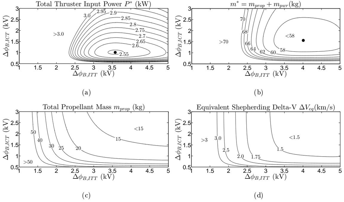
**Fig. 8** Representations of a) total thrusters input power; b) optimizable EPS dedicated mass; c) total propellant mass; and d) equivalent shepherding delta-V.
