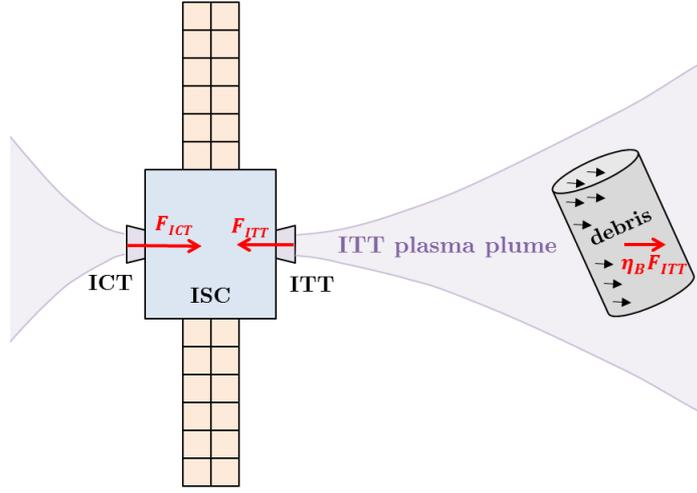
**Fig. 1 Schematic of the ion beam shepherd concept**
