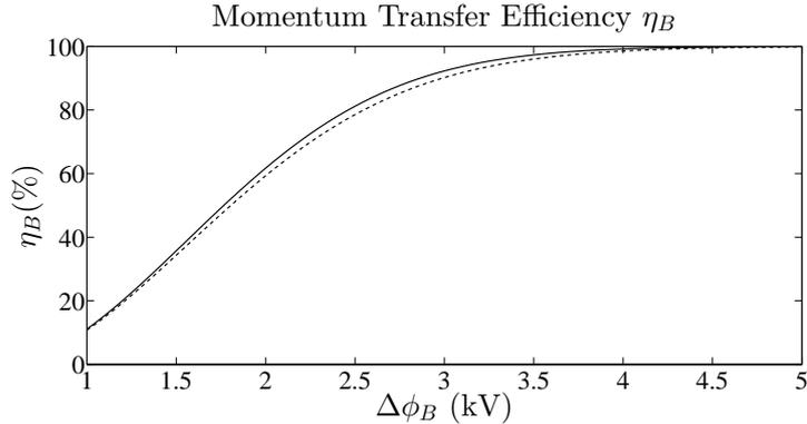
**Fig. 6** Momentum transfer efficiency versus  $\Delta\phi_B$ , for  $R_0 = 7$  cm (solid line) and 25 cm (dashed line).
