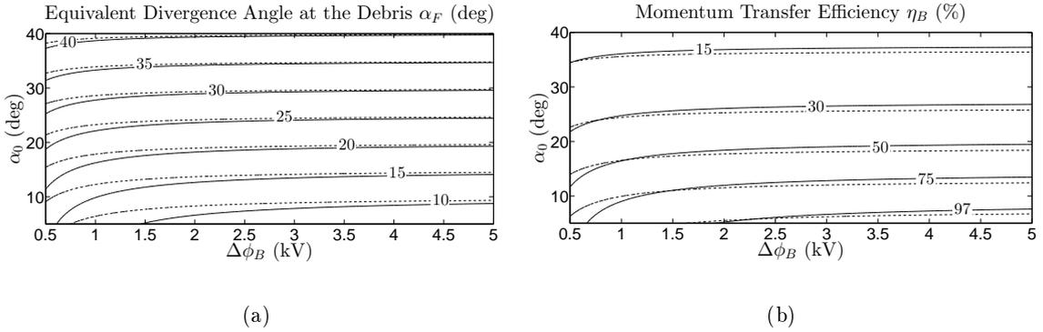
**Fig. 5 Representations of a) equivalent conical divergence angle and b) momentum transfer efficiency, for  $R_0 = 7$  cm (solid line) and 25 cm (dashed line).**
