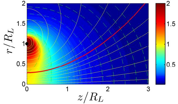
Figure 1: Meridian plane of the magnetic field created by a current loop placed at  $r = R_L$ . Yellow lines are field lines. The line chosen as nozzle outer line has been highlighted in red. Green, dashed lines represent  $B$ -constant lines. The background color shows the magnetic field intensity relative to  $B_S$ , its value at the origin.
