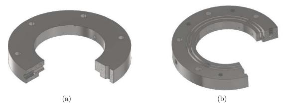
Figure 3.5: (a) CAD section view of the propellant injector v1. (b) CAD section view of the propellant injector v2, a fitting lid (not visible in the figure) positioned at the top of the injector encloses the channels preventing leaks.
