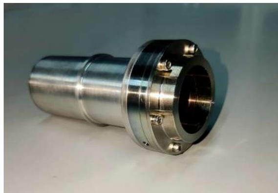
Figure 3.4: Photo of the assembly of the thruster aluminum waveguide and plasma chamber.
