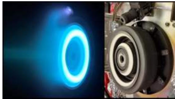
Fig. 1.1. Picture from NASA's Jet Propulsion Laboratory (JPL) of a HET. On the left, the plasma during operation emitting a blue light characteristic of xenon plasma, on the right the thruster turned off [1].
