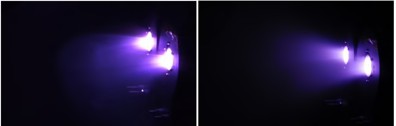
(a) Two ECR sources cluster in operation with 15 sccm Krypton and 100 W. MF ARCH magnetic topology ( I_{BC} = 11 A and I_{MN} = 8.5 A) in use. (b) Two ECR sources cluster in operation with 15 sccm Krypton and 100 W. MF SAME magnetic topology ( I_{BC} = 11 A and I_{MN} = 8.5 A) in use.
