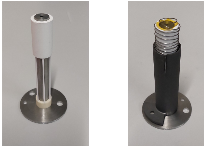
(a) Bird cage heater sleeve assembly (b) Heater filament assembly
