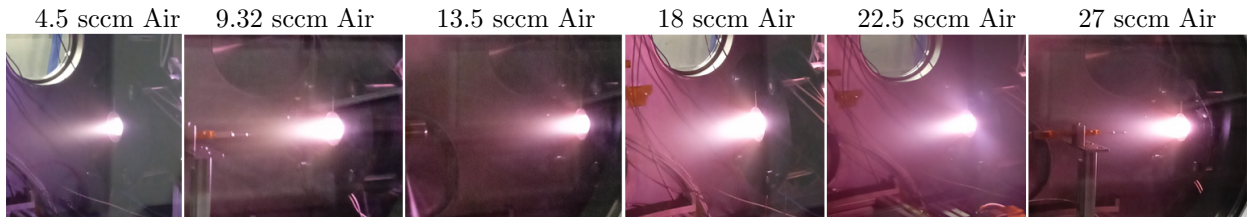
Figure 5. Plasma plume of the HPT operating with air under different conditions (from left to right: 4.5, 9.32, 13.5, 18, 22.5 and 27 sccm Air).
