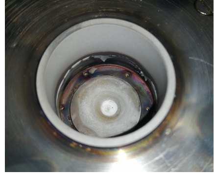
Fig. 4 Eroded central ceramic
